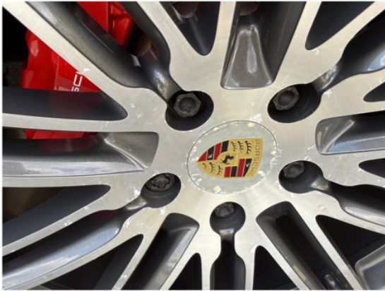
Felge hinten links Oxidation
